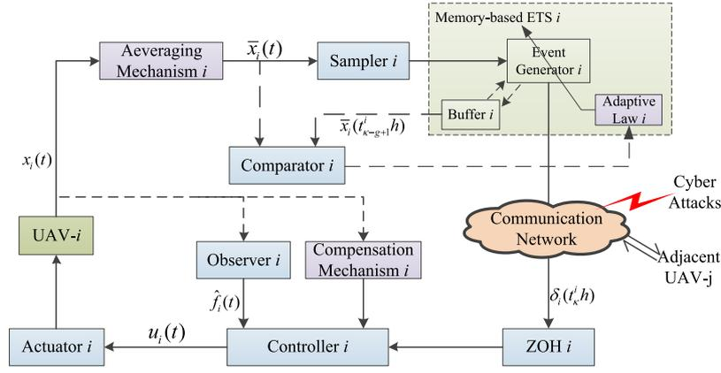
Fig. 1. Structure of the memory-based consensus control for the  $i$ th UAV against deception attacks.
