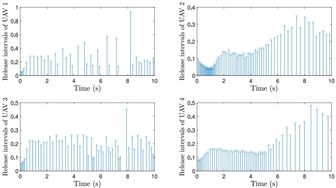
Fig. 8. Release instants and triggering intervals of followers with METS under deception attacks.
