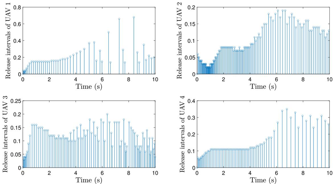
Fig. 11. Release instants and triggering intervals of followers with fixed threshold under deception attacks.
