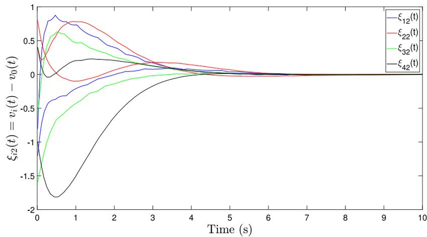
Fig. 4. Tracking errors of the velocity for UAVs.
