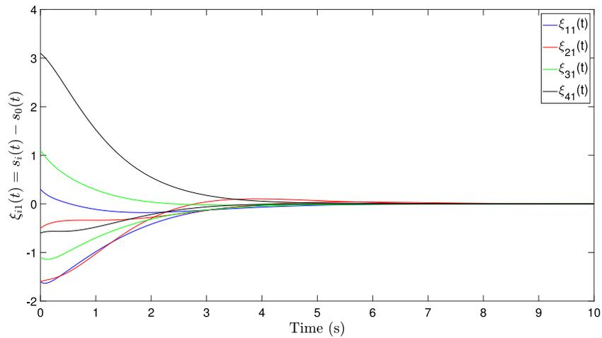
Fig. 9. Tracking errors of the displacement for UAVs with fixed threshold.
